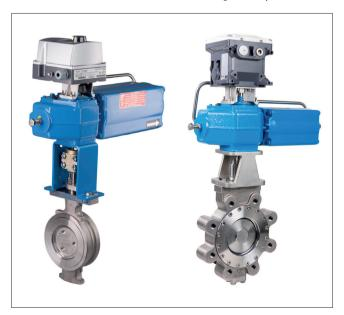
High-cycle constructions for both the valve and actuator are offered as a standard for PSA units. Our predefined constructions provide the necessary bearing and soft goods to meet the required life cycle for our Jamesbury 800-series butterfly valves. Our high-cycle Neles B-series actuators also come equipped with the correct bearing material and design to withstand millions of cycles as standard.
