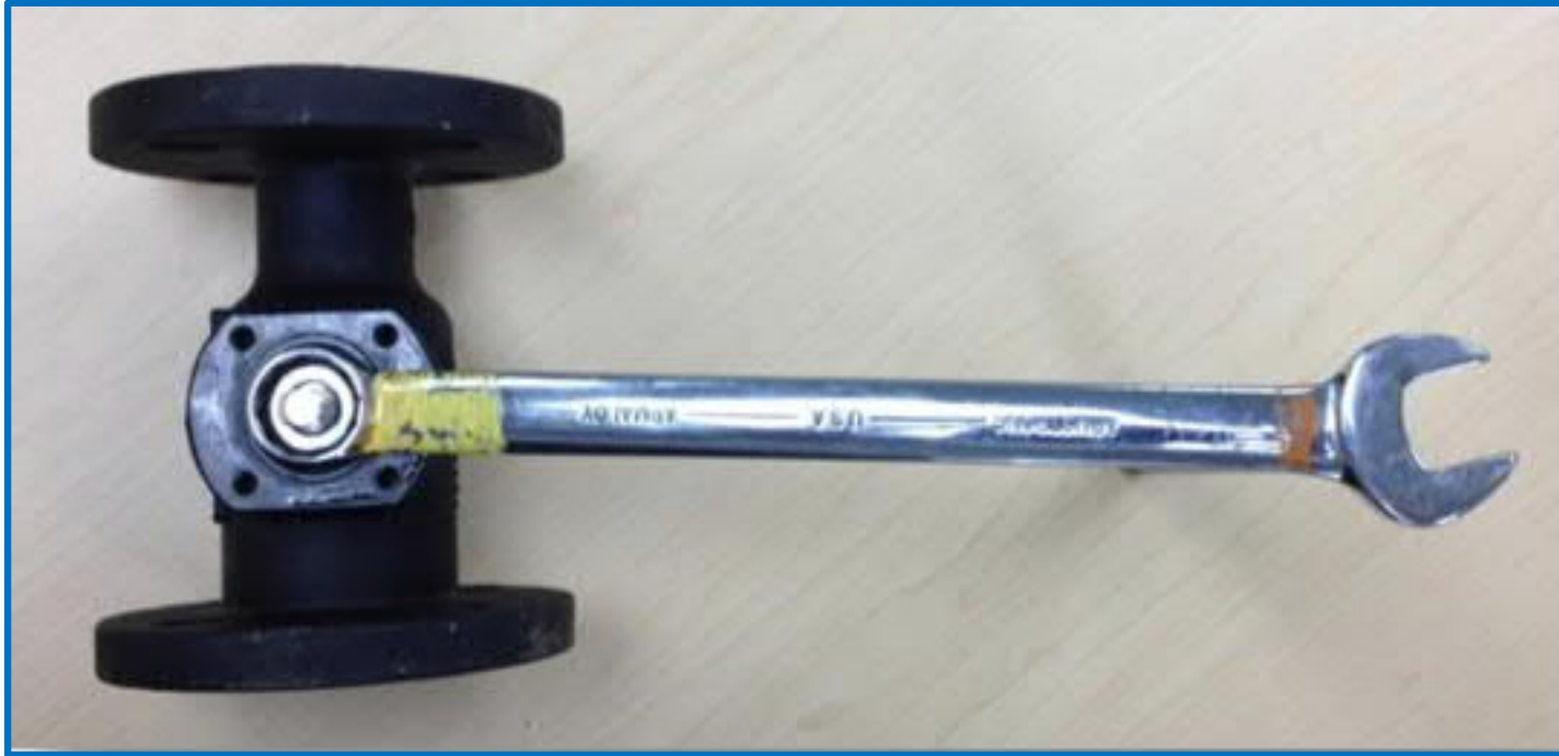
Competitor valves using nuts on stem to compress packing require a wrench size that will easily crush the seal when tightened
