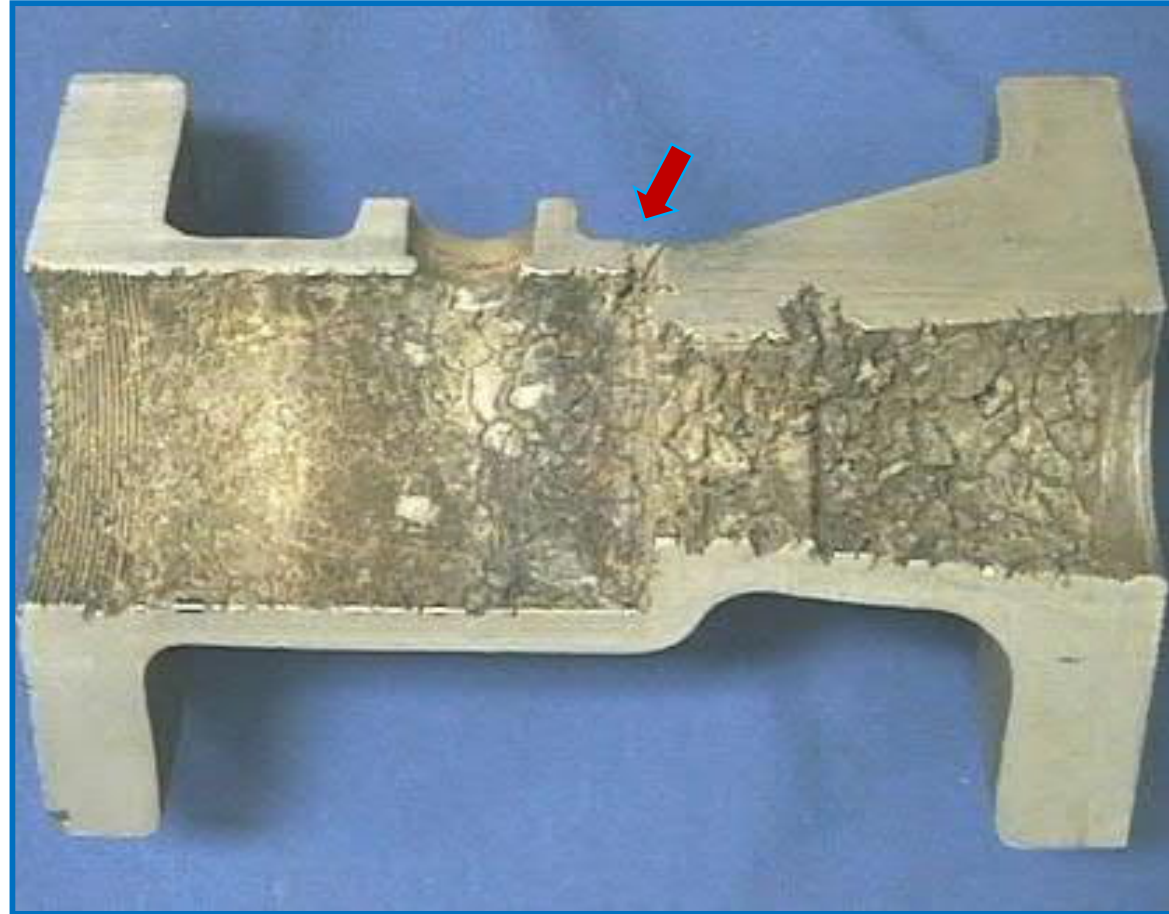
If not properly annealed, stainless steel in Nitric acid, corrosion in just 3 weeks penetrated through the wall
